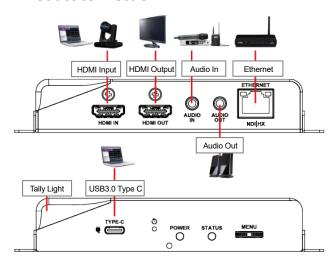
\*OIP-N40E supports PoE (IEEE 802.3af) network switches or USB-C power supply
